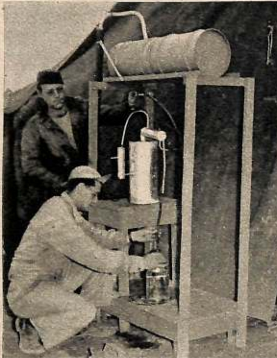
S/Sgt. Charles Lewis (rear) and T/Sgt. Robert J. Simpkins with a still they made for a squadron in Sardinia for distilling battery water. They used oil drums and a plane heating unit.
