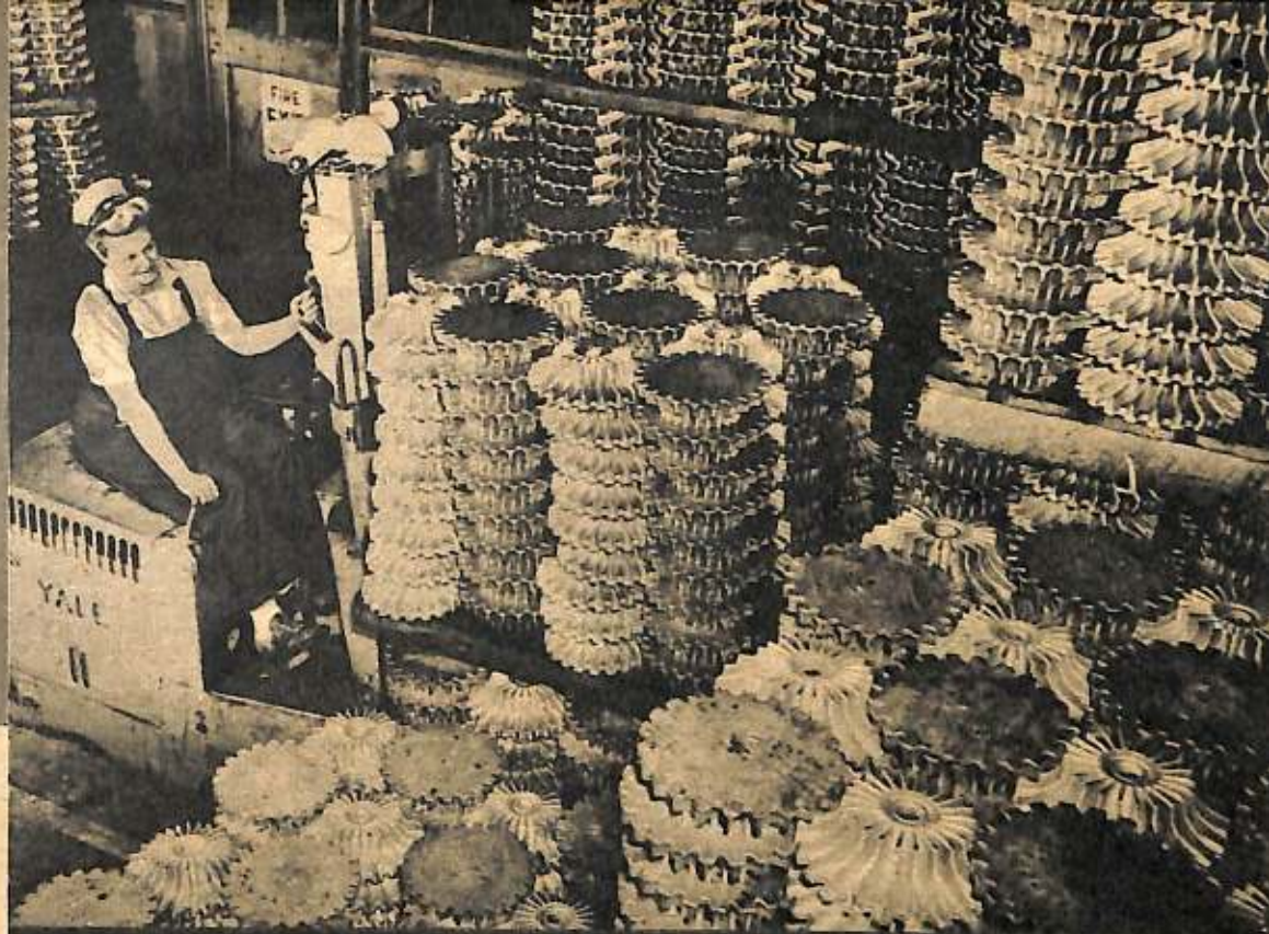
A new device for superchargers are these "impellers" which revolve 20,000 times a minute to give high altitude flying another boost and more power.
