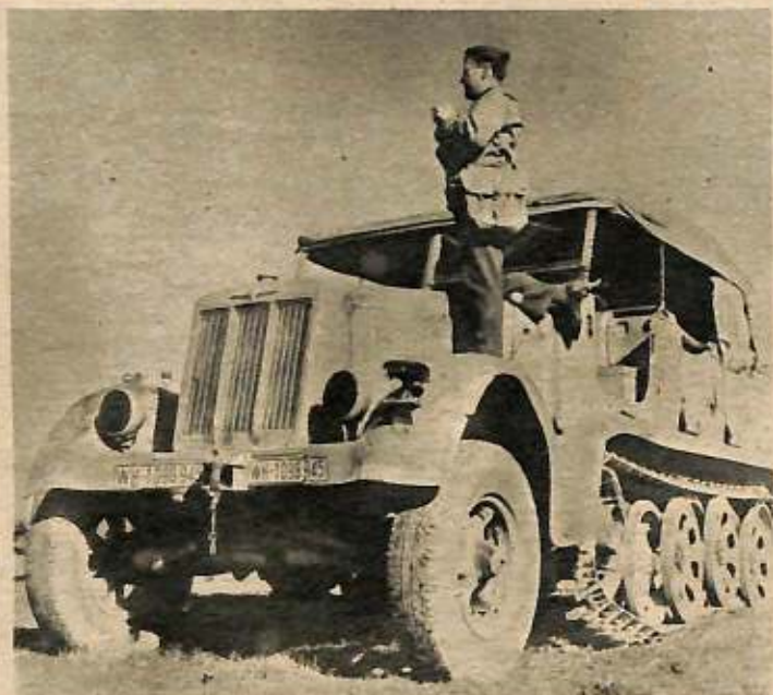
This is the German eight-ton half-track personnel carrier and prime mover. It has a passenger capacity of 12 men and is used as the standard tractor for the 88-mm dual-purpose gun.
