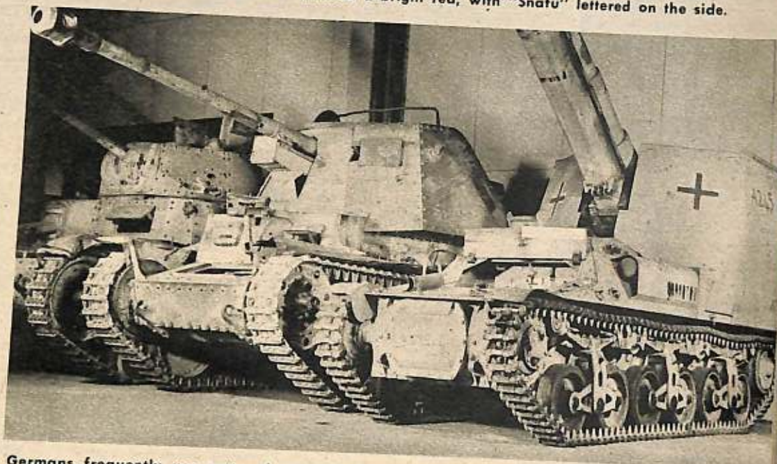
Germans frequently use captured material intact or convert it to suit their own purposes. In the foreground above is a German 15-cm howitzer mounted on a French Lorraine medium tank chassis. To its right is a German 75-mm gun on a Czech medium tank chassis.
