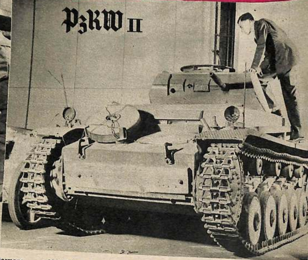
with a 20-mm auto-cannon and one 7.92-mm machine gun. In the close-up at left is shown the quarter-elliptic springing of bogies which has been replaced in newer German models by a torsional-suspension system. This PzKW II came into Aberdeen painted a bright red, with "Snafu" lettered on the side.
