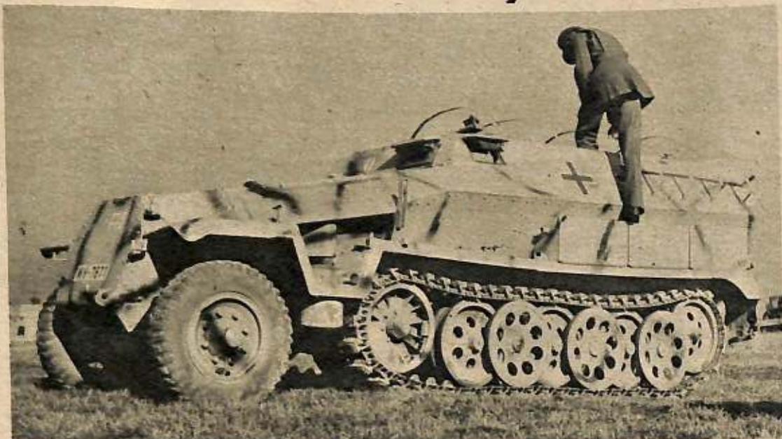
The German armored half-track personnel carrier is a six-cylinder, 100-horsepower job with a maximum speed of 40 mph. It carries two MG34 machine guns. This vehicle has a coffin-shaped body, and carries 10 men on two longitudinal seats. One machine gun is mounted to the right of the eleventh man, the driver, whose visibility is limited to two small glassed-in slots as shown above.
