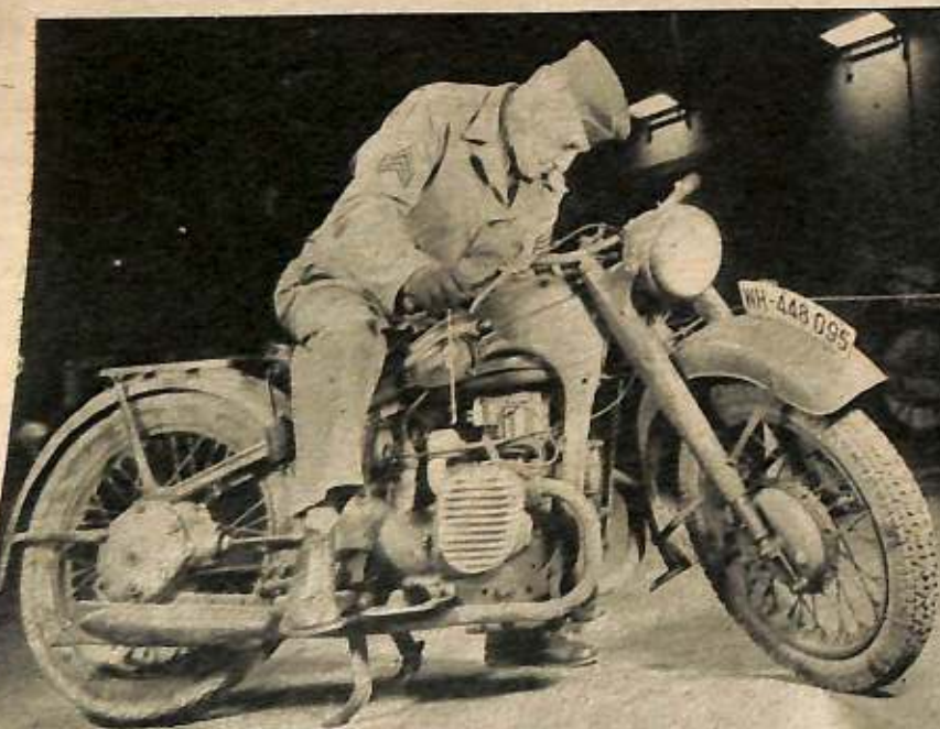
The Nazi BMW motorcycle has an opposed horizontal twin engine, driving the rear wheel by a shaft instead of a chain. Unlike most European models it has a hand gear shift similar to conventional U. S. models.
