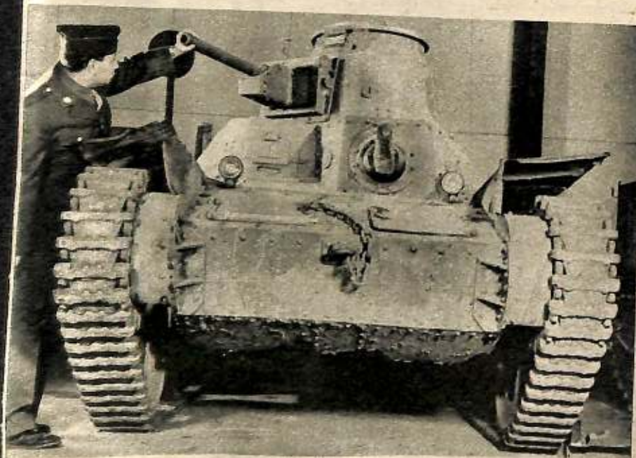
JAPANESE light tank, model 1935, pictured above and right, was built in October 1941 and was captured last summer in the Aleutians. Like most Japanese equipment, it performs better than it looks. It has a six-cylinder air-cooled 250-horsepower Diesel engine which moves its eight-ton weight at 22 mph. It is armed with a 37-mm cannon and two 7.7 machine guns. Note the old-style riveting of armor plate throughout.
