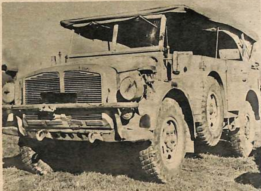
The spare wheel on each side of the chassis of this German command and reconnaissance car turns freely to prevent bellying on rough ground. It has a V-8 engine, four-wheel drive, and can do 45 mph. There is no armament.
