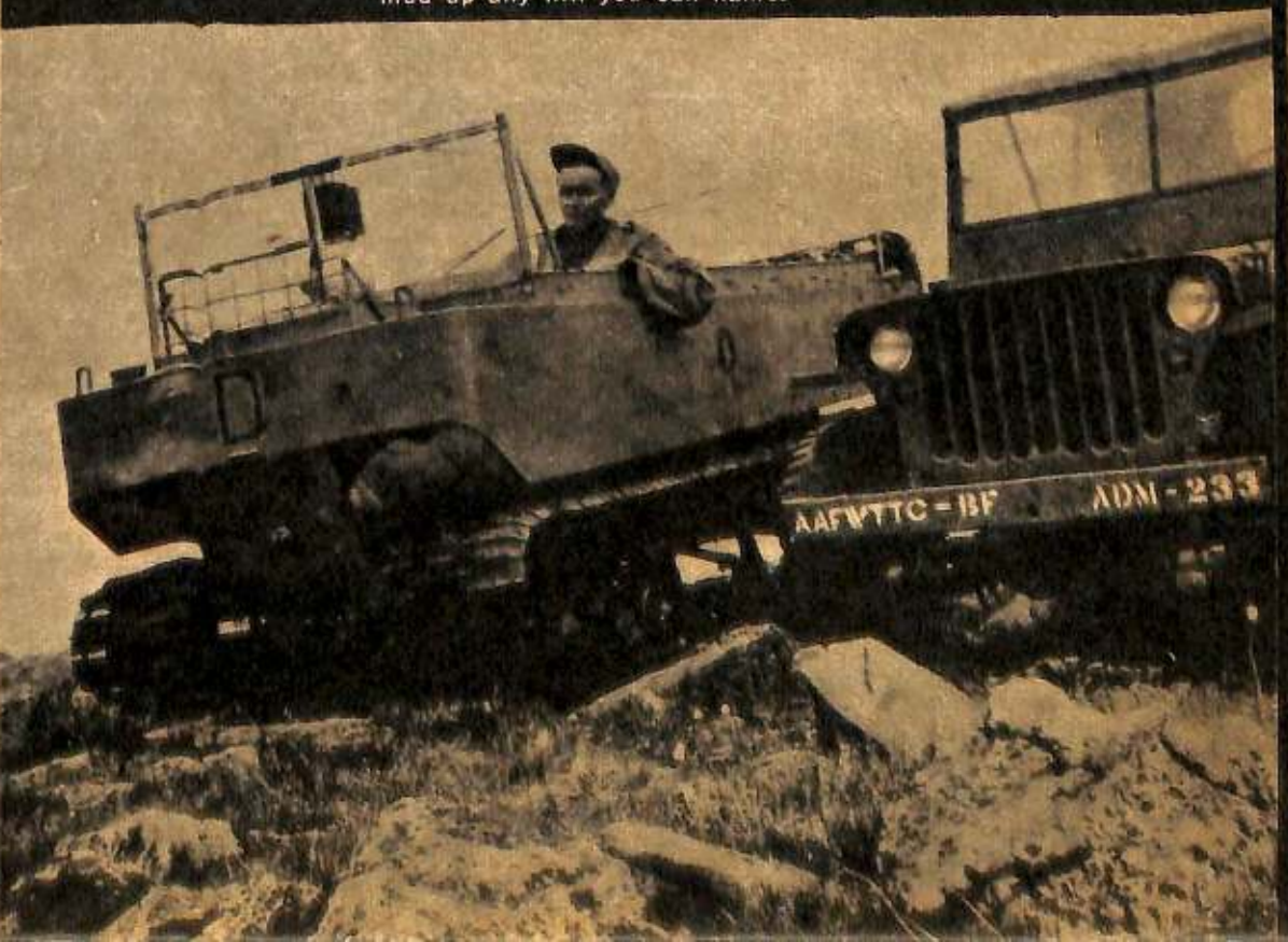
Jinx Falkenburg, the film lovely, poses a pretty problem for tire thieves. The crossed-steel gage on the wheel stops grab artists from removing either tire or rim. Interesting, isn't it—and she? Below, we unveil the jeep's new sister—the U.S. M-29. This water baby on tracks can tote GIs or cargo of 1,200 pounds through mud up any hill you can name.
