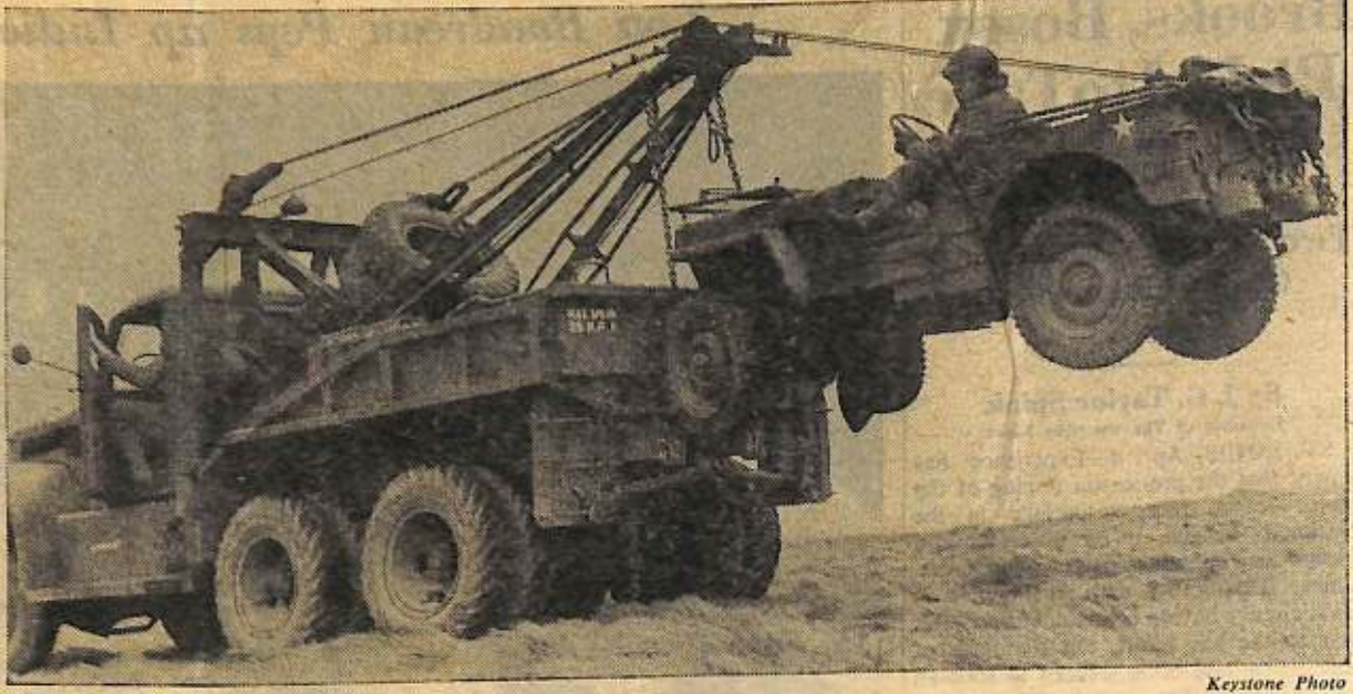
A power-driven crane from an 11-ton U.S. wrecker truck picks up a 3,200-pound peep to carry it from a field during a battle exercise in England by American Ordnance men.
