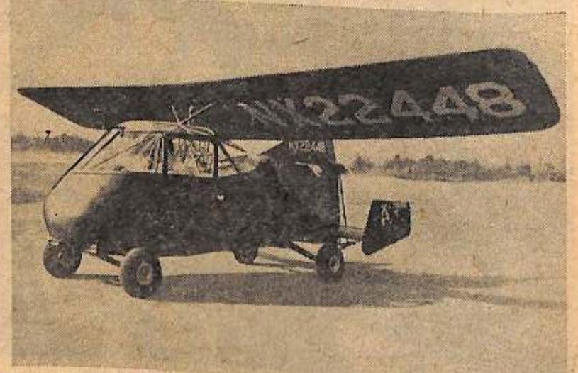
CONTROLLABLE WINGS, seen on this plane, may revolutionize control methods on small aircraft. Testers believe that controllable wings would eliminate ailerons, elevators and rudders on small planes.
