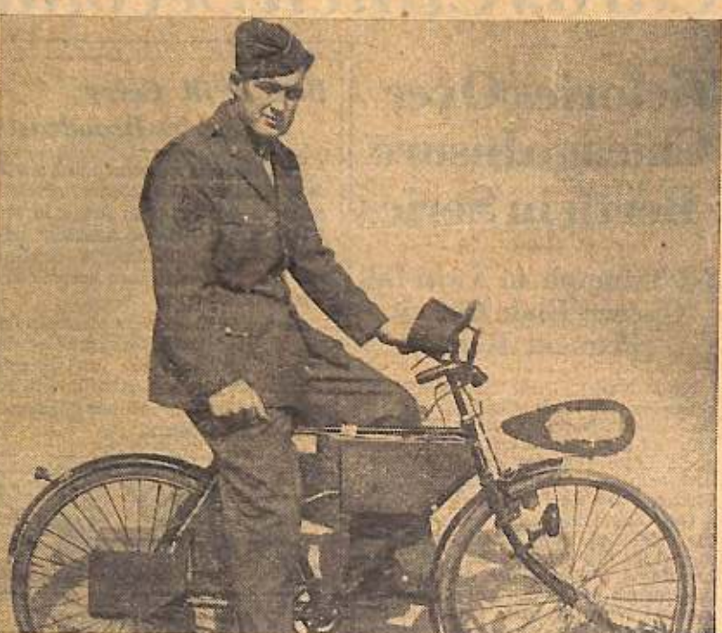
T/3 Earl Kirkaby, of Dayton, N.D., built himself this "bikarola" radio out of odds and ends of materials he found around his station workshop. The four-tube super-heterodyne has a loop antenna which makes his bicycle look like something out of Buck Rogers. The radio runs on a six-volt chargeable battery. A home-made converter replaces the usual B battery.
