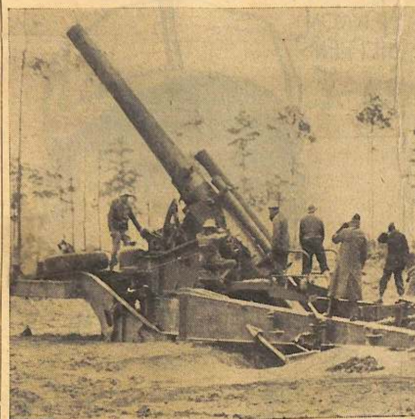
This is our new 240mm. howitzer, the M-1, as described in the Field Artillery Journal. It is more mobile and more powerful, and even more accurate than its 1918 counterpart. It travels in two loads on high-speed trailers. Less digging is required for its emplacement, and this is speeded by a clumpshell bucket. This is attached to the battery crane, which also eliminates the time-consuming jacking of loads into position.
